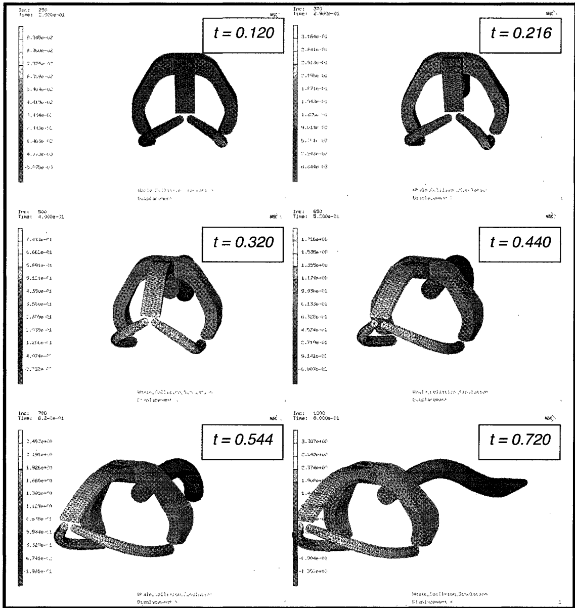
Figure 5.16. 5-knot direct impact collision progression, deformation of skeleton.
