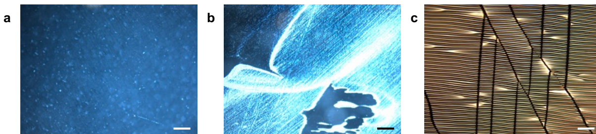
Figure S12. (a) Optical micrograph of 30- \mu\text{m} -thick PDMS film adhered to a bulk PDMS substrate by molecular glue without silicon tetrachloride vapor deposition. (b) Optical micrograph of delamination of the PDMS membrane stretched to 130% elongation. (c) Optical micrograph of a 250- \text{\AA} -thick gold film deposited on the PDMS membrane surface and stretched to 30% elongation (all scales = 150 \mu\text{m} ). Samples were stretched in the horizontal direction.
