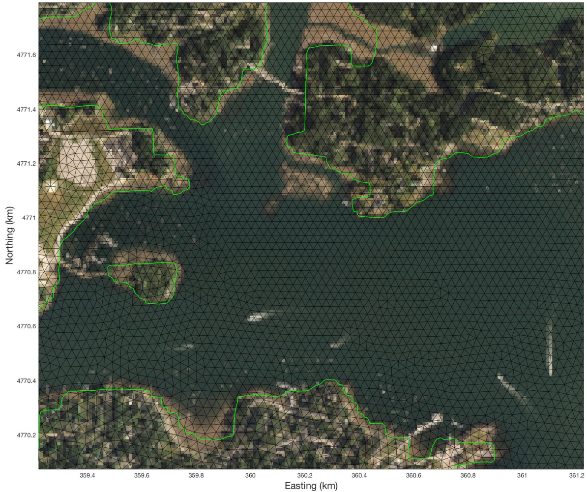
Figure 7. Close up of portion of the grid, showing fine scale resolution near boundary. The shoreline at mean sea level is shown with the green line.
