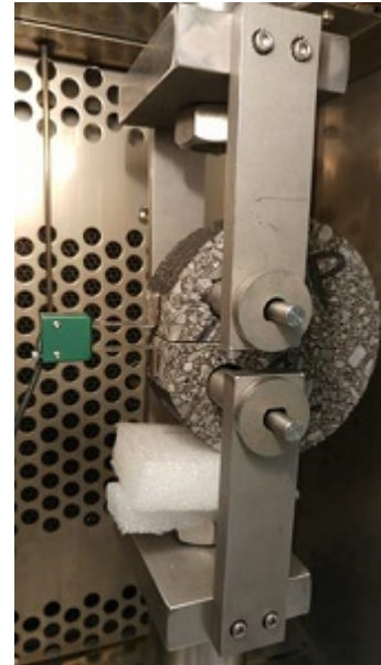
DCT testing fixture used at UNH. The vertical bars pull on the specimen, generating tensile forces at the end of the notch cut into the asphalt concrete.
