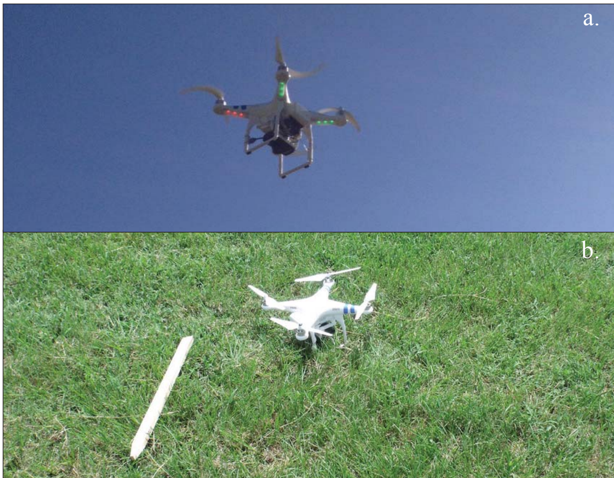
Figure 7. The DJI Phantom 2 quadrotor unmanned aerial vehicle used in the aerial survey work at the M. S. Roberts site (41HE8): a, in the air; b, stationary.
