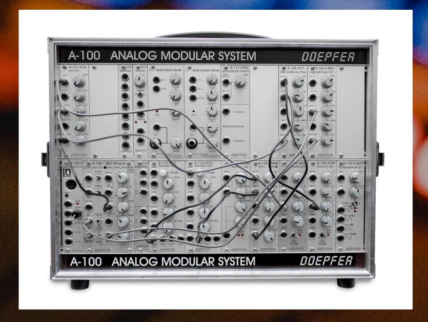
What is a Modular Synth?: An electronic device (or program) that generates a signal which can be altered one parameter at a time using specialized controllers—or "modules." There are many types of modules that can affect different parts of a signal such as oscillators, filters, amplifiers, and many others.
