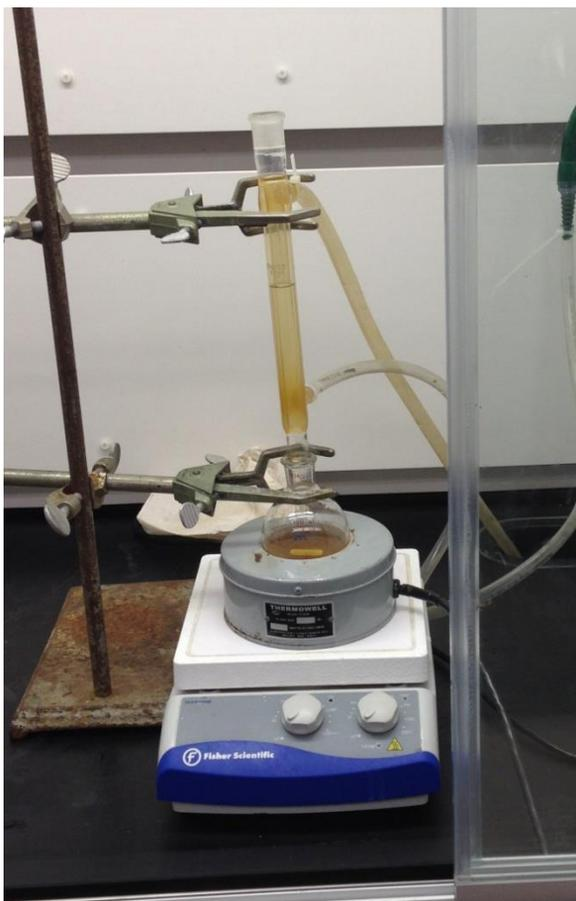
***Figure 9: Conventional-heated reaction apparatus***
