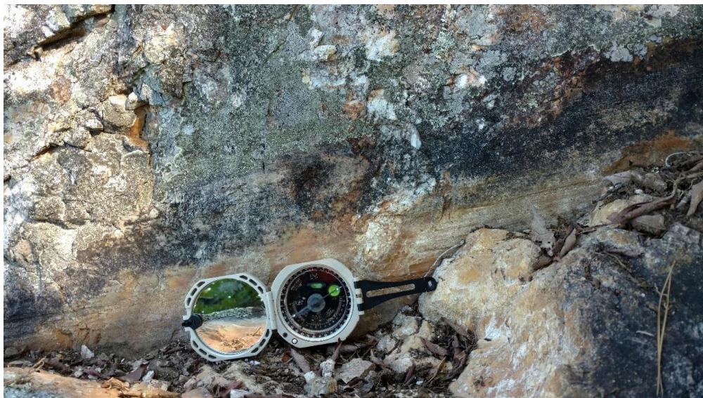
Figure 4.34. Right-lateral strike-slip fault with slickenlines at Stop 111 (see Figure 4.31 for location). Brunton for scale.
