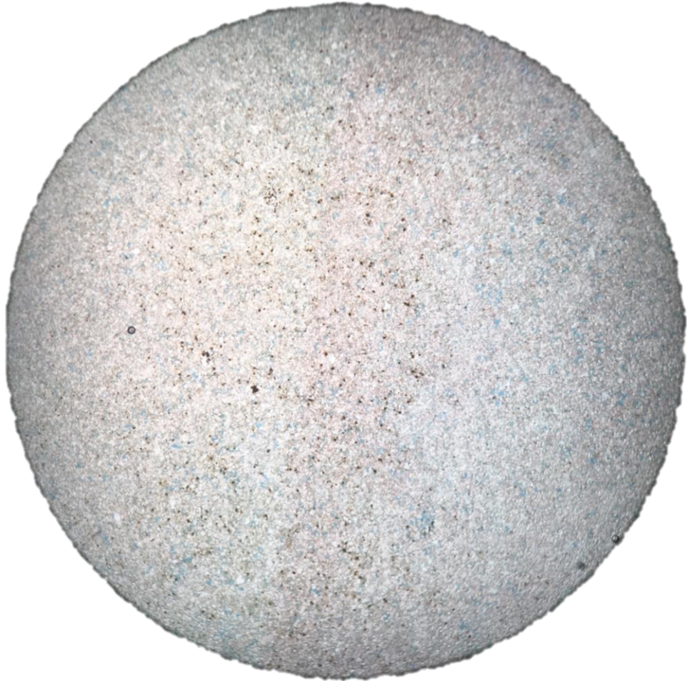
Figure 112. Sample A09-011 Section 6 Glen Rose Formation Unit 2 Magnification is 4x with field of view is 1 cm. Plain light thin section of micrite (Folk) mudstone (Dunham). A 300-point count graph thin section, 60% micrite, 30% quartz, 10% porosity.
