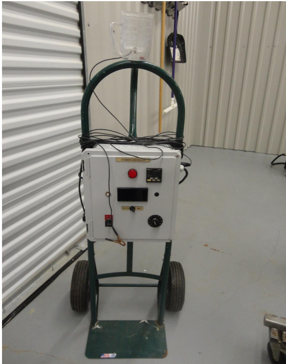
Figure 5: Step (1) in the processing procedure. The Pulsed DC Poultry Stunner from Executrol Systems
