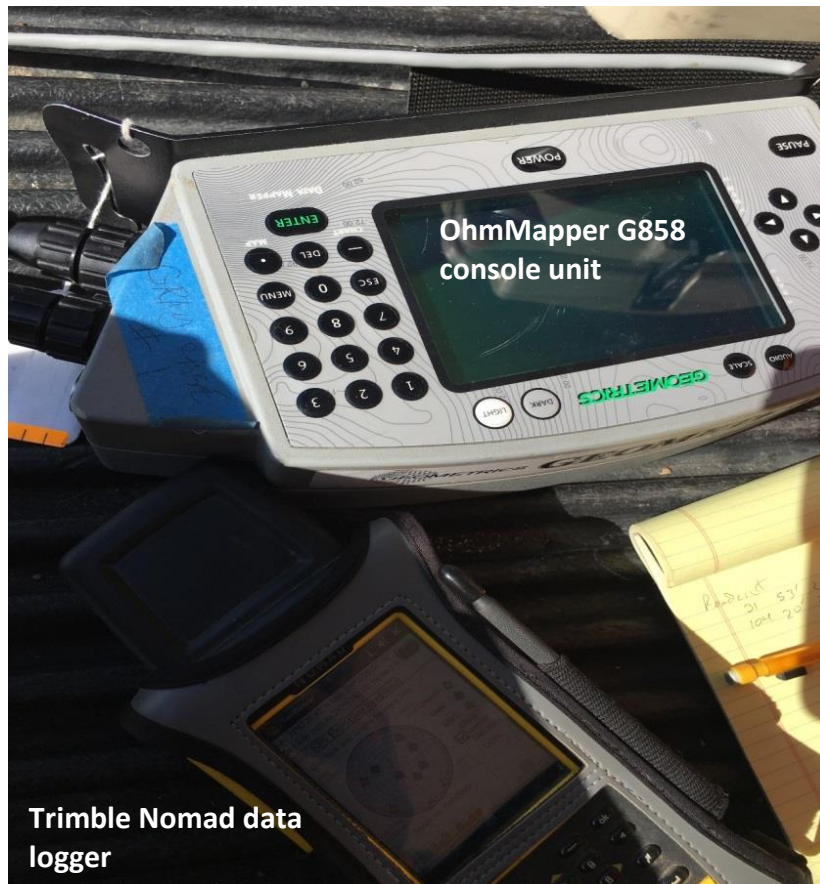
Figure B2. Image of the OhmMapper G858 resistivity meter on the top portion of the photo, and the Trimble Nomad 900 Series GPS data logger in the bottom portion of the photo.
