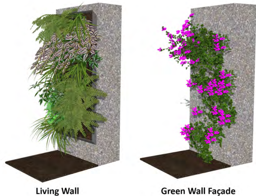
Figure 26: Living wall and green wall façade diagram
