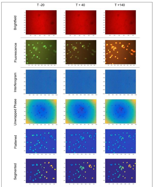
**Figure 5. Example of HSLCI image processing pipeline steps.** Images shown are of the same location at three different time points. Brightfield and fluorescent images were collected with a Basler color CCD camera and did not undergo processing after acquisition. Interferograms were collected by a Phasics QWLSI camera and were subsequently converted into unwrapped phase images, flattened, and segmented to yield mass data for single cells.
