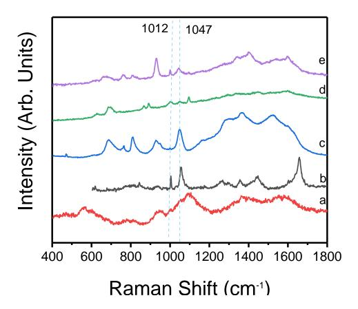
**Figure 3.8** (a) Raman spectrum of 20-HETE (pure compound) along with SERS spectra of **20-HETE** acquired with 10  $\mu$ L aliquots of (b) 1 mM, (c) 1  $\mu$ M, (d) 1 nM, and (e) 1 pM dilutions. Thin films of citrate-coated Ag nanoplatelets were used as the SERS substrates.
