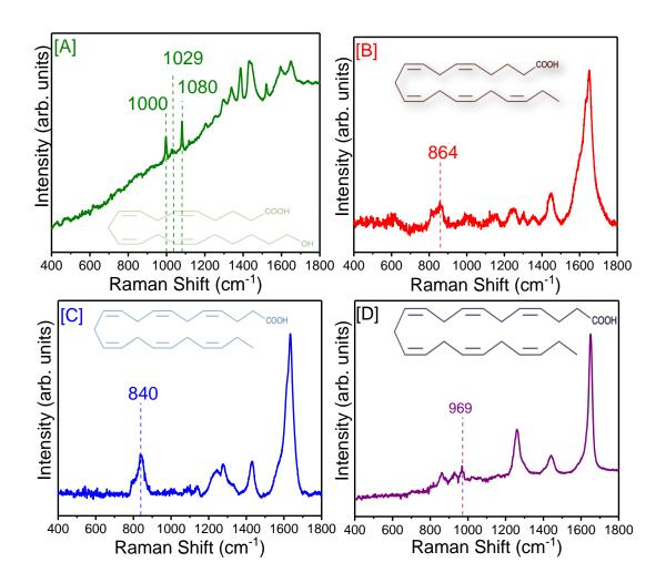
**Figure 4.6.** Normal Raman spectra of pure lipids and their molecular structures: (A) 20-Hydroxyeicosatetraenoic acid (20-HETE), (B) arachidonic acid (AA), (C) docosahexaenoic acid (DHA), and (D) eicosapentaenoic acid (EPA).
