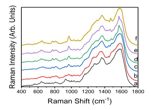
**Figure 3.9** The 20-HETE burning study was done on citrate covered triangular silver nanoplatelets, with spectra record at the following time intervals: (a) 400s, (b) 800s, (c) 1700s, (d) 2600s, (e) 3500s and (f) 4400s.
