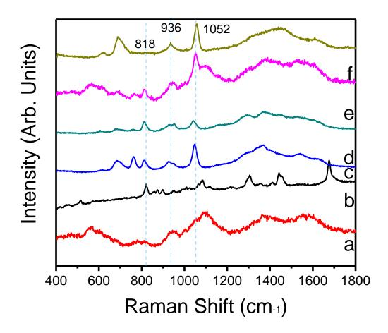
Figure 3.6 (a) Raman spectrum of pure 6-keto postaglandin-f1 $\alpha$  along with SERS spectra of 6-keto prostaglandin-f1 $\alpha$  acquired with 10  $\mu$ L aliquots of (b) 1 mM, (c) 1  $\mu$ M, (d) 1 nM, and (e) 1 pM dilutions. Thin films of citrate-coated Ag nanoplatelets were used as the SERS substrates.
