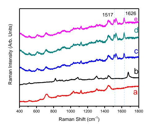
**Figure 3.4** (a) Raman spectrum of pure **6-keto prostaglandin-f1α** along with SERS spectra of **6-keto prostaglandin-f1α** acquired with 10 μL aliquots of (b) 1 mM, (c) 1 μM, and (e) 1 nM dilutions. Octanethiol-coated Au nanoparticle films were used as SERS substrates.
