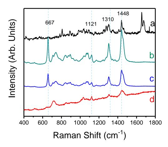
**Figure 3.5** (a) Raman spectrum of pure **Thromboxane B2** along with SERS spectra of **Thromboxane B2** acquired with 10  $\mu$ L aliquots of (b) 1 mM, (c) 1  $\mu$ M, and (e) 1 nM dilutions. Octanethiol-coated Au nanoparticle films were used as SERS substrates.
