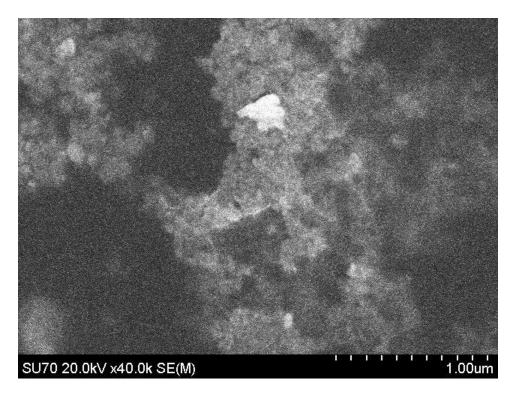
**Figure 4.2.** SEM image of the Ag nanoplatelet substrate show polydispersity and aggregation of nanoparticles.
