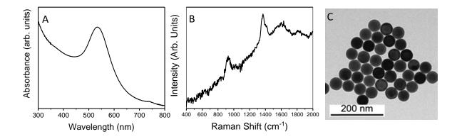
**Figure 3.2** (A) UV-Vis spectrum with 530 nm plasmon, (B) Raman spectrum with multiple interfering functional groups which would make lipid detection less definitive and (C) TEM image of glutathione capped gold nanoparticles, used to determine a 30nm average particle size and that the synthesis produced homogenous particles.
