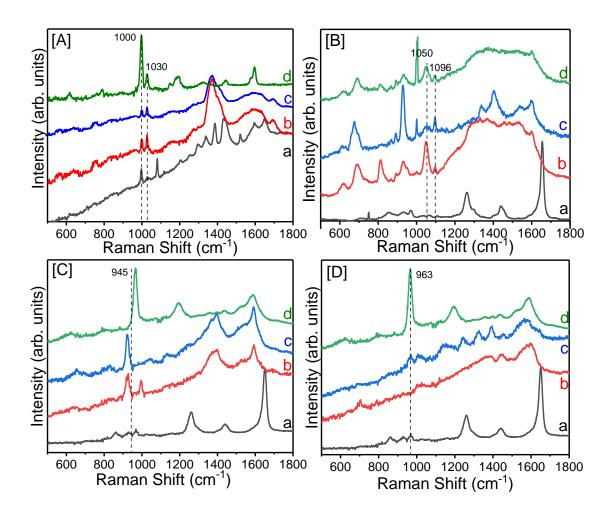
**Figure 4.7.** (a) Raman spectra and (b) 1 μM SERS, (c) 1 nM SERS, and (d) 1 pM SERS spectra of (A) 20-HETE, (B) AA, (C) DHA and (D) EPA. The dash lines of each spectrum indicate the significant peaks that were used for qualitative analysis corresponding lipids in mixing studies.
