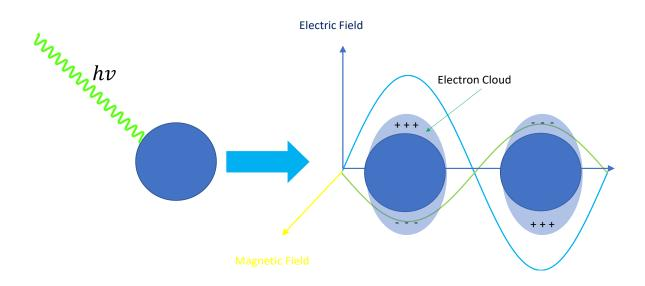
Figure 2.3 Diagram of localized surface plasmon resonance.
