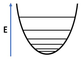
Figure 2.2 Vibrational energy well diagram
