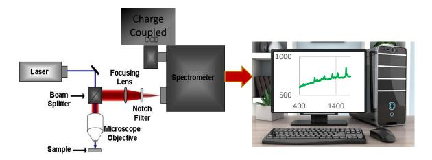
Figure 2.1 Raman spectrometer instrumentation.
