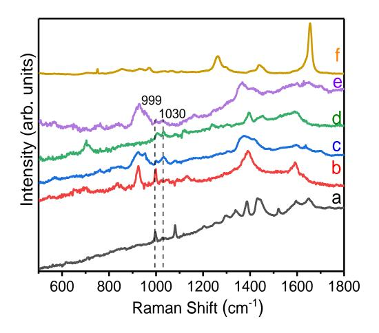
**Figure 4.8.** (a) Raman spectrum of 20-HETE along with SERS spectra of (b) 1 nM AA and 1 nM 20-HETE, (c) 1 nM AA and 100 pM 20-HETE, (d) 1 nM AA and 10 pM 20-HETE, (e) 1 nM AA and 1 pM 20-HETE and (f) Raman spectrum of AA. These data suggest that 20-HETE is still detectable in the presence of AA with three orders of magnitude higher concentration. The highlighted region indicates the prominent 20-HETE peaks.
