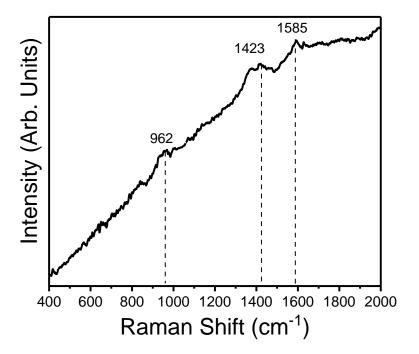
**Figure 4.1.** Representative SERS spectrum of the Ag nanoplatelet substrate deposited on glass showing that the region between 1000-1100 cm<sup>-1</sup> does not interfere with 20-HETE peaks in this region of the spectrum.
