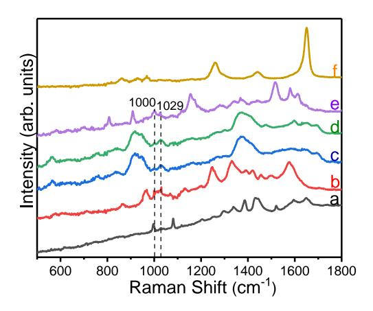
**Figure 4.10.** (a) Raman spectrum of 20-HETE along with SERS spectra of (b) 1 nM EPA and 1 nM 20-HETE, (c) 1 nM EPA and 100 pM 20-HETE, (d) 1 nM EPA and 10 pM 20-HETE, (e) 1 nM EPA and 1 pM 20-HETE and (f) Raman spectrum of EPA. This data suggests that 20-HETE is detectable in the presence of EPA with three orders of magnitude higher concentration. The highlighted region indicates the prominent 20-HETE peaks.
