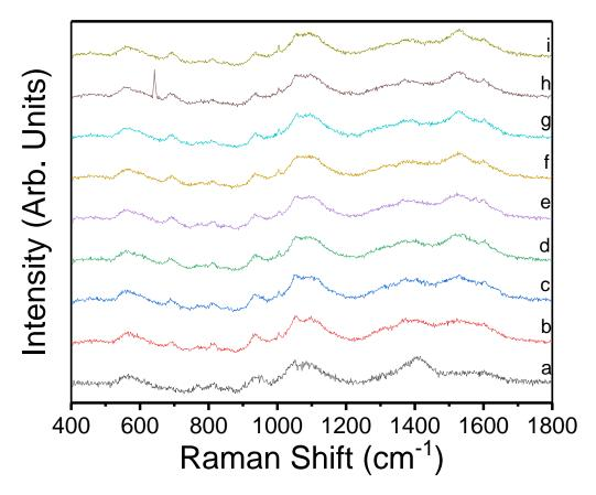
**Figure 3.3** Burning study of platelet substrate. In this study, a 532.11nm laser emitting at 20 μW was shined on the substrate to test stability of the substrate under the laser at (a) 1 min, (b) 12 min, (c) 18 min, (d) 24 min, (e) 30 min, (f) 42 min, (g) 48 min, (h) 54 min, (i) 60 min
