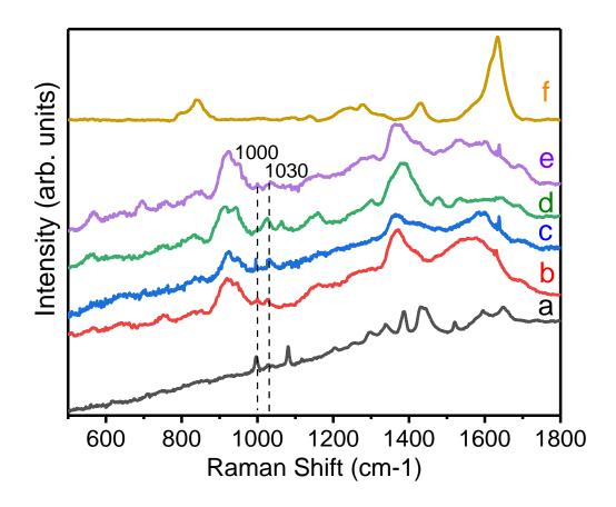
**Figure 4.9.** (a) Raman spectrum of 20-HETE along with SERS spectra of (b) 1 nM DHA and 1 nM 20-HETE, (c) 1 nM DHA and 100 pM 20-HETE, (d) 1 nM DHA and 10 pM 20-HETE, (e) 1 nM DHA and 1 pM 20-HETE and (f) Raman spectrum of DHA. These data suggest that 20-HETE is detectable in the presence of DHA with three orders of magnitude higher concentration. The highlighted region indicates the prominent 20-HETE peaks.
