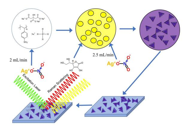
**Scheme 4.1.** A schematic illustration of the synthesis of Ag triangular nanoplatelets for SERS detection of bioactive lipids.
