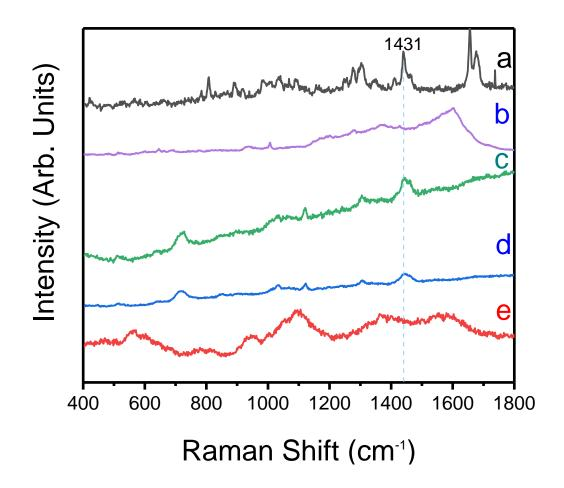
**Figure 3.7** (a) Raman spectrum of TXB2 (pure compound) along with SERS spectra of **TXB2** acquired with 10  $\mu$ L aliquots of (b) 1 mM, (c) 1  $\mu$ M dilutions. Thin films of citrate-coated Ag nanoplatelets were used as the SERS substrates.
