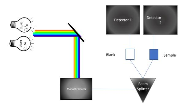
Figure 2.4 UV-Vis operational schematic.
