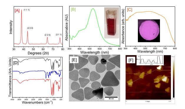
**Figure 4.4.** (A) Powder XRD pattern, (B) Solution-state and (C) solid-state UV-Visible absorbance spectra and (D) FT- IR spectra of (a) Ag nanoplatelets along with (b) trisodium citrate and (c) poly(styrenesulfonate) surfactants used in the synthesis Ag particles. (E) A representative TEM image of Ag nanoplatelets used in the SERS detection of bioactive lipids. (F) An AFM image of Ag nanoplatelets drop-casted on glass substrates including depth profile.
