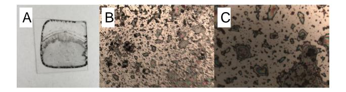
**Figure 4.3.** Photographs showing visible images of drop-cased Ag nanoplatelet substrate with (A) 1X, (B) 10X, and (C) 100X magnification showing randomly distributed and aggregated particles. Despite polydispersity and aggregation on the surface of the coverslip, the Intensity of UV-Vis transmission spectra maintained the same pattern and within 10% transmission for any given wavelength, determined by 5 collected spectra on visible different spots.
