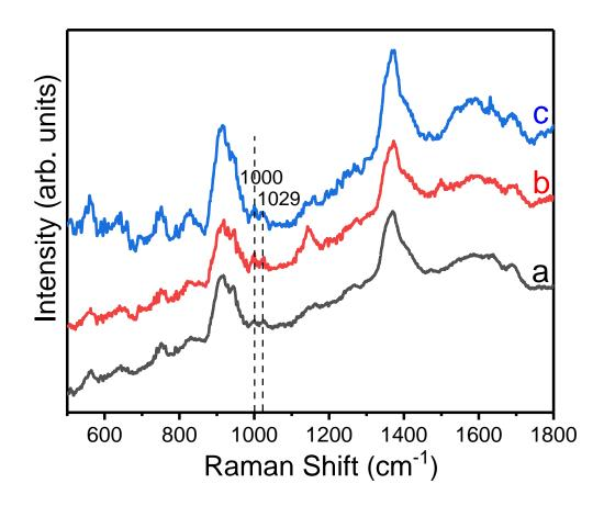
**Figure 4.11.** (a-c) SERS spectra of a mixture of 4.56 μM AA, 821.1 nM DHA, 129 nM EPA, and 86.7 nM 20-HETE, demonstrating that at biologically relevant concentrations of these lipids, 20-HETE can still be reproducibly detected and differentiated from other lipids. The highlighted region indicates the prominent 20-HETE peaks.
