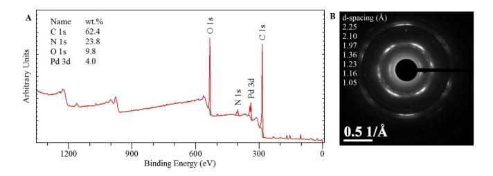
Figure 5-3 (A) atomic survey on the surface of Pd/G catalyst measured by x-ray photoelectron spectroscopy. (B) SAED shows the crystalline structure of Pd. SAED was performed in an area of about 100 nm<sup>2</sup>. The right side of Fig. 4a shows the SAED pattern and the measured d-spacing
