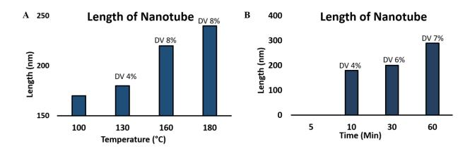
Figure 6-3 Fig (A) shows the length of the carbon nanotube as a function of and temperature after 10 mins of the microwave irradiation. Fig (B) shows the length of the carbon nanotube as a function of time after the microwave irradiation at 130 °C.
