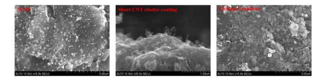
Figure 6-5 Ni@GNP generated using ball milling and domestic microwave.
