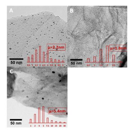
Figure 5-2 TEM image and particle size distribution of Pd/graphene catalyst fabricated by (**A**) co-reduction method, (**B**) SEA method and (**C**) Post solventless microwave heating method (SEA-MW).
