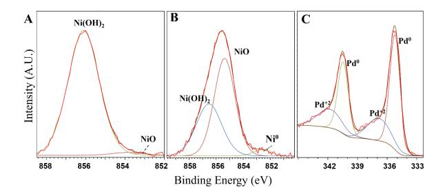
Figure 6-6 XPS result shows the different Ni and Pd peaks in the sample (A) Ni@GNP BM, (B)Ni@GNP BM-KMW2MIN and (C) Pd@CNT-GNP Hydrazine and Microwave reduction
