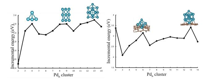
Figure 2-8 Incremental energies of free and supported  $Pd_n n=1-14$  clusters.
