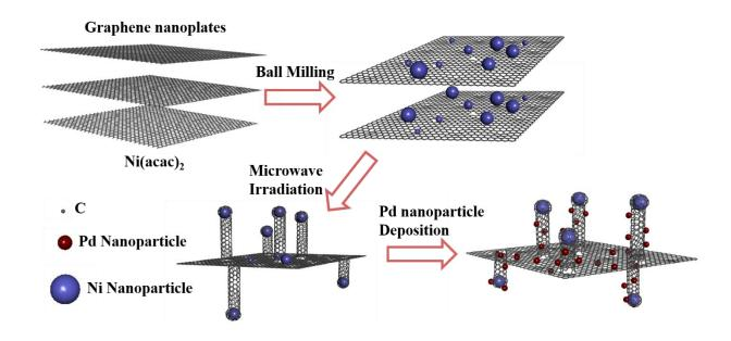
Figure 6-1 The strategy of the synthesis of the CNT/GNP hybrid and immobilizing the Pd nanoparticles on the 3-D CNT/GNP substrate.
