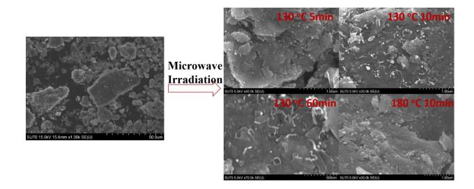
Figure 6-2 Left figure shows the Ni-graphene mixture after ball milling. Right figures show the growth of carbon nanotube on the graphene under microwave irradiation.
