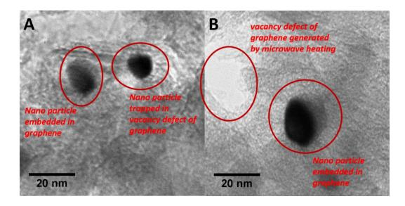
Figure 5-4 TEM images show isolated vacancy defect site on the graphene sheet, vacancy site that accommodating Pd nanoparticles, as well as Pd nanoparticle embedded in the graphene. Catalyst generated via solventless microwave method.
