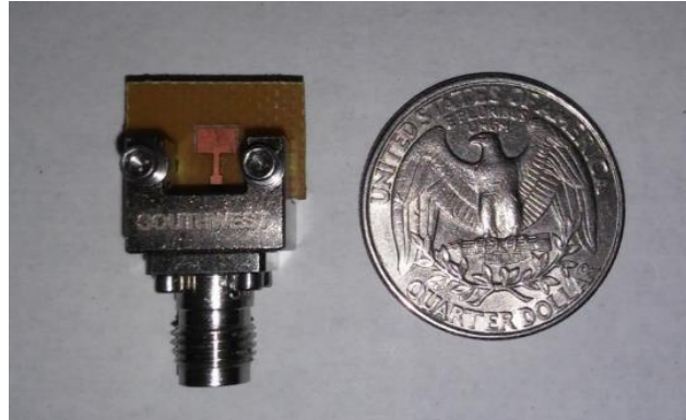
Figure 7: Fabricated antenna with the end launch connector
