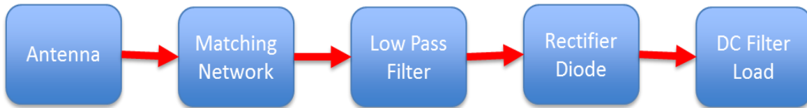
Figure 1: Main components of the rectenna. From left to right: antenna, low pass filter, rectifier diode, and DC filter output.
