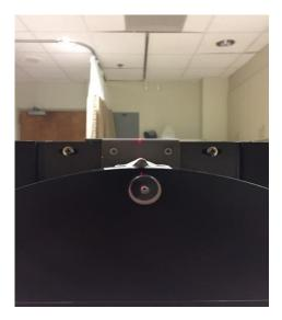
Fig. 4.6 An experimental setup for scatter signal measured is shown. A tungsten rod was placed on top of calibration phantom
