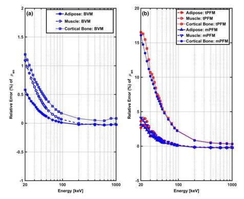
Fig. 5. Relative estimation error of energy-absorption coefficients for adipose, muscle and cortical bone by (a) BVM and (b) vPVM and tPFM models. [Color figure can be viewed at wileyonlinelibrary.com]
