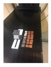
Fig.4.10. A collimator assembly <sup>98</sup> and stacks of AI and Cu are shown
