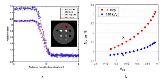
Fig 5.11 The ESFs from 90 kVp and 140 kVp of cortical bone is shown on (a). The two crosses in (b) correspond to MTF derived from ESF curves in (a). Each point on the tradeoff curves corresponds to Gaussian smoothing kernel in a range of 0 mm to 1.5 mm.
