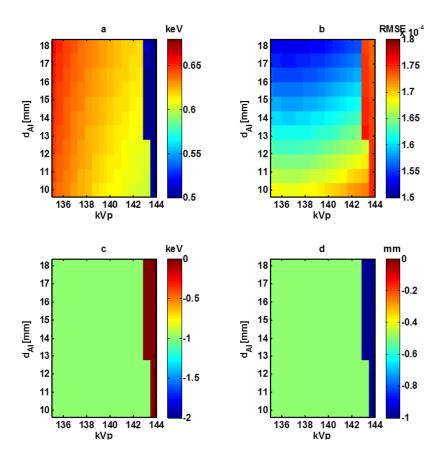
Fig.4.19 Comparisons of derived spectrum and independently simulated reference spectra for nomial 140 kVp with inherent filtration of aluminum ranging from 10 mm to 18 mm for the noisy  $QF_{P,model}$  The differences of mean energy (a), RMSE (b), kVp(c), and d<sub>Al</sub> (d) are shown, respectively. Each pixel on the figures corresponded to the discrenpance for each candidate of reference spectrum
