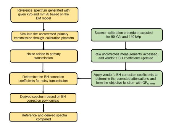
Fig.4.9. Flowchart of the procedure of uncertainty analysis of spectrum. A Poisson noise was added to primary transmission from reference spectrum, which yielded an updated set of BH polynomial correction coefficients. The derived spectrum was also compared against reference spectrum.
