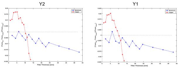
Fig. 4.12. The transmission comparisons for spectra of 140 kVp at Y1 and Y2 through filters
