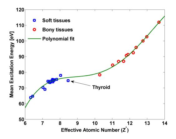
Fig.2.3 The polynomial relationship <sup>55</sup> between Z\* and mean excitation energy was implemented in the VCU tPFM. The fit of R<sup>2</sup> is 0.9603. Data for 34 soft tissues and bony tissues are shown.
