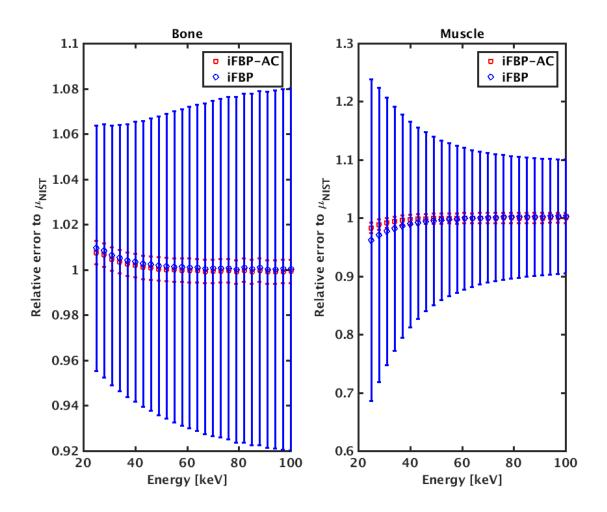
Fig. 5.17 Mean errors with 95% uncertainties error bars in estimated linear attenuation coefficient of ICRU bone and muscle tissue are shown for both iFBP and iFBP-AC algorithms, respectively.
