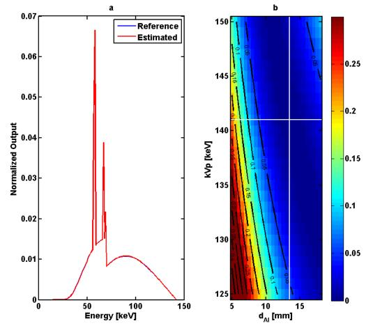
Fig.4.14 Comparison of derived spectrum and independent measured spectrum for 140 kVp of Y2 shown in (a), and the white cross in (b) correspoding to parameters for specifying a spectrum based on BM model.
