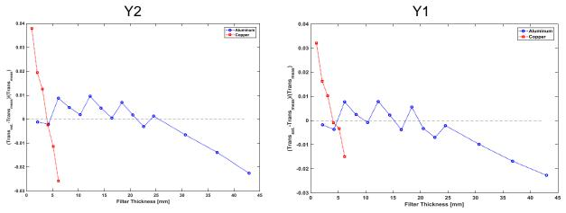
Fig. 4.11. The transmission comparisons for spectra of 90 kVp at Y1 and Y2 through Al and Cu filters
