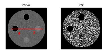
Fig. 5.12 Reconstructed c<sub>1</sub> images from noisy sinogram. A profile line across inserts 2 and 4 is shown. The noise levels in BVM muscle insert 2 for iFBP-AC and iFBP are 0.009 and 0.125, respectively. The true c<sub>1</sub> value of insert is 0.87. The view window is set [0.75 1]
