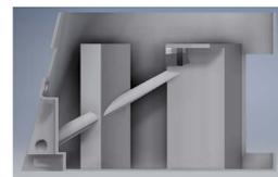
Cross-sectional view showing the chute in which the pills will travel from the ring to the tray..
