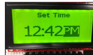
Set Time menu where the user can set the current time to calibrate the device.
