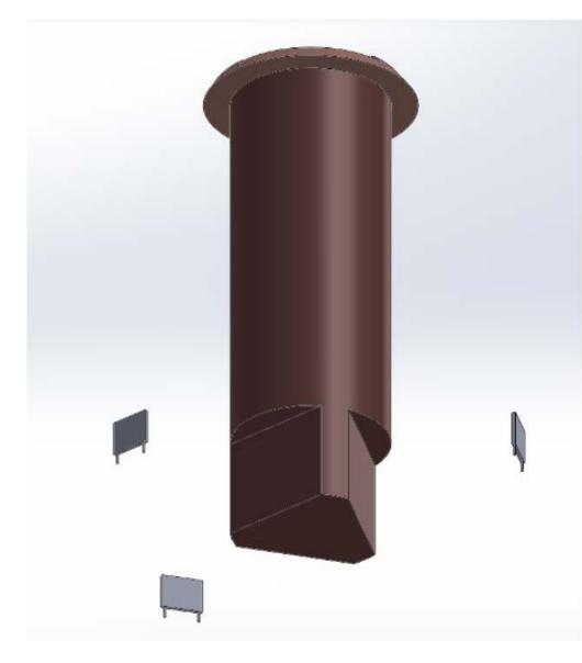
Once a vibration is detected the sensor transmits a wireless signal to a solar powered gateway above ground. The gateway then has the capability to transmit that signal to the user.
