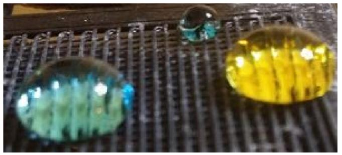
As the mesh is not a solid surface, it leaves direct contact between the air and water on either side. Depending on the ratios of concentration in these two fluids, diffusion can transfer oxygen across this interface. If oxygen content on the air side of the barrier decreases, by respiration or some other process, it may be possible for that consumed oxygen to be resupplied by the water.
