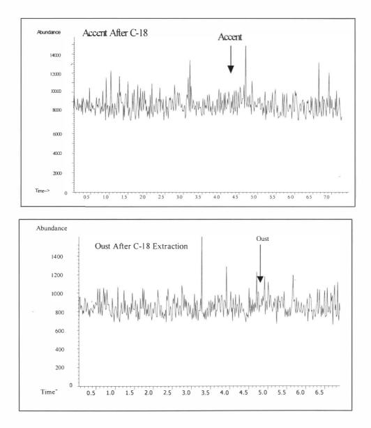
Figure 31. TIC of Accent and Oust After C-18 Extraction. Arrows indicate the expected retention times of the herbicides in the liquid chromatograms.
