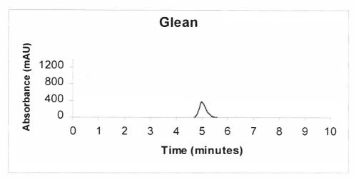
Figure 25. Liquid Chromatogram of Glean The flow rate was 0.4 mL/min, the mobile phase was (75:25) ACN/H2O, both containing 0.05% HAc. The column was a Phenomenex LUNA C-18(2), 150 x 4.60 mm, 5  $\mu$ m particle size column. UV detection was at 254 nm. Concentration was 100ug/mL.
