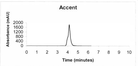
Figure 21. Liquid Chromatogram of Accent The flow rate was 0.4 mL/min, the mobile phase was (75:25) ACN/H2O, both containing 0.05% HAc. The column was a Phenomenex LUNA C-18(2), 150 x 4.60 mm, 5  $\mu$ m particle size column. UV detection was at 254 nm. Concentration was 100ug/mL.
