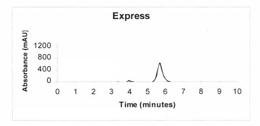
Figure 24. Liquid Chromatogram of Express. The flow rate was 0.4 mL/min, the mobile phase was (75:25) ACN/H2O, both containing 0.05% HAc. The column was a Phenomenex LUNA C-18(2), 150 x 4.60 mm, 5  $\mu$ m particle size column. UV detection was at 254 nm. Concentration was 100ug/mL.
