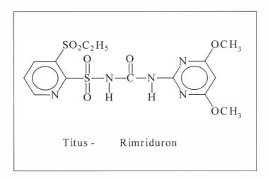
Figure 7. Structure of the sulfonylurea herbicide, Titus
