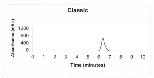
Figure 23. Liquid Chromatogram of Classic. The flow rate was 0.4 mL/min, the mobile phase was (75:25) ACN/H2O, both containing 0.05% HAc. The column was a Phenomenex LUNA C-18(2), 150 x 4.60 mm, 5  $\mu$ m particle size column. UV detection was at 254 nm. Concentration was 100ug/mL.
