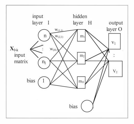
Figure 12. Feed-Forward, Back-Propagation Artificial Neural Network. The ANN in this figure consists of three layers, an input layer, a hidden layer, and an output layer.
