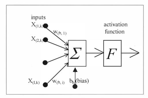
Figure 13 - The Artificial Neuron - A signal,  $X_{lxK}$ , at the input layer is connected to hidden neuron h and is multiplied by a weight  $w_{hxi}$ , where h is the neuron number and i is the input node number.
