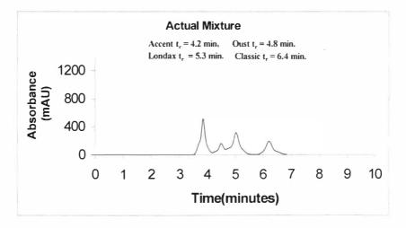
Figure 30. Actual Chromatogram of a Mixture of Accent, Oust , Londax, and Classic. The flow rate was 0.4 mL/min, the mobile phase was (75:25) ACN/H2O, both containing 0.05% HAc. The column was a Phenomenex LUNA C-18(2), 150 x 4.60 mm, 5  $\mu$ m particle size column. UV detection was at 254 nm. Concentration was 100ug/mL.
