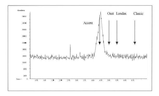
Figure 48. TIC of the Mixture After the Silica Extraction.
