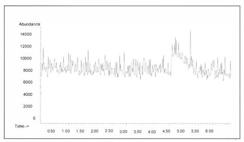
Figure 38. TIC of Blank after SAX Extraction.
