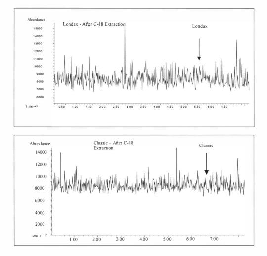
Figure 32. TIC of Londax and Classic After C-18 Extraction. Arrows indicate the expected retention times of the herbicides in the liquid chromatograms.
