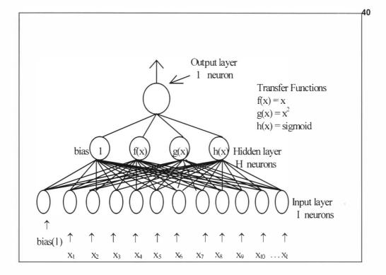
Figure 17. Schematic Diagram of an ANN
