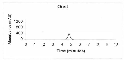
Figure 28. Liquid Chromatogram of Oust. The flow rate was 0.4 mL/min, the mobile phase was (75:25) ACN/H2O, both containing 0.05% HAc. The column was a Phenomenex LUNA C-18(2), 150 x 4.60 mm, 5  $\mu$ m particle size column. UV detection was at 254 nm. Concentration was 100ug/mL.
