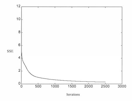
Figure 20. Plot of the Sum-Squared Error during Training. For a feed-forward, back-propagation ANN with 47 input neurons, 6 hidden neurons, and 8 output neurons
