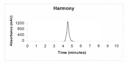
Figure 26. Liquid Chromatogram of Harmony. The flow rate was 0.4 mL/min, the mobile phase was (75:25) ACN/H2O, both containing 0.05% HAc. The column was a Phenomenex LUNA C-18(2), 150 x 4.60 mm, 5  $\mu$ m particle size column. UV detection was at 254 nm. Concentration was 100ug/mL.
