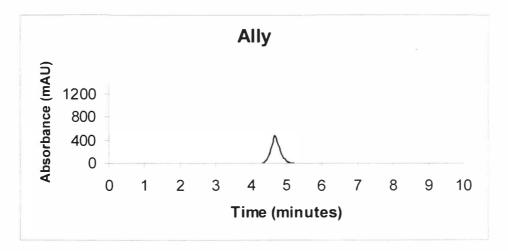
Figure 22. Liquid Chromatogram of Ally. The flow rate was 0.4 mL/min, the mobile phase was (75:25) ACN/H2O, both containing 0.05% HAc. The column was a Phenomenex LUNA C-18(2), 150 x 4.60 mm, 5  $\mu$ m particle size column. UV detection was at 254 nm. Concentration was 100ug/mL.
