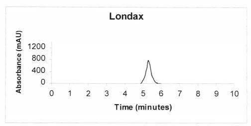
Figure 27. Liquid Chromatogram of Londax. The flow rate was 0.4 mL/min, the mobile phase was (75:25) ACN/H2O, both containing 0.05% HAc. The column was a Phenomenex LUNA C-18(2), 150 x 4.60 mm, 5  $\mu$ m particle size column. UV detection was at 254 nm. Concentration was 100ug/mL.
