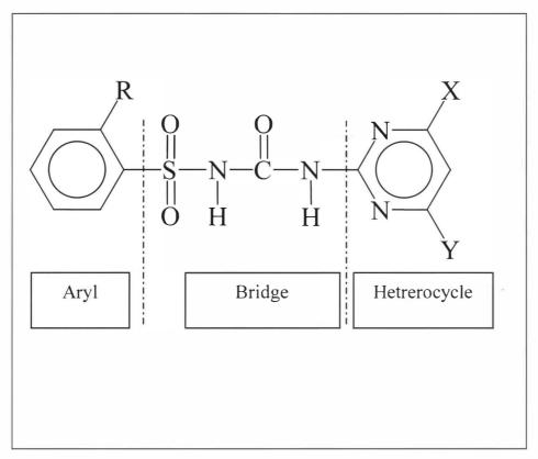
Figure 2. General Structure – Sulfonylurea Herbicides, composed of three segments, an aryl segment, a heterocyclic ring segment, and a bridge connecting the two.
