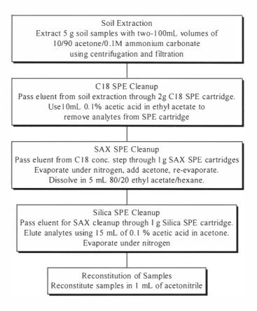
Figure 19. Extraction Procedure Flowchart. The flow chart diagrams the extraction through the use of three different solid-phase extraction cartridges, a C-18 SPE, a SAX-SPE, and a Si-SPE.
