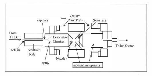
Figure 18. The Particle Beam Interface. The interface consists of a nebulizer, a desolvation chamber, and a momentum separator.
