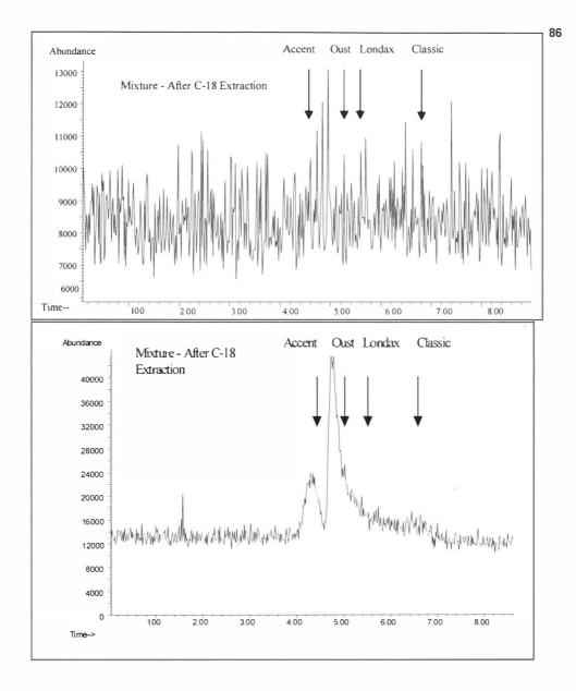
Figure 33. TICs of the Mixture After the C-18 and SAX Extractions. Arrows indicate the expected retention times of the herbicides in the liquid chromatograms.
