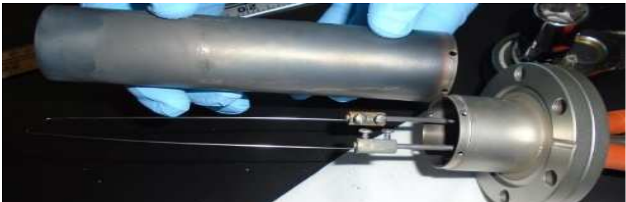
Figure 2.5. Image of hot wire element and gas inlet taken during maintenance for filament replacement.
