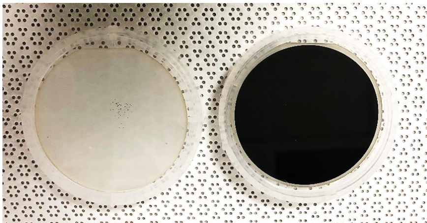
Figure 13. GaN with no coating (left) and GaN with backside coated with Ti (right).
