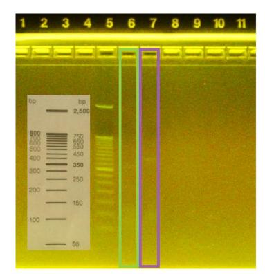
Figure 6. Gel electrophoresis image of PCR amplicons after the cleavage detection enzyme has been applied to the samples.
