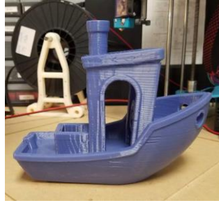
Figure 4-2: Finished Result of Freestanding Print Test
