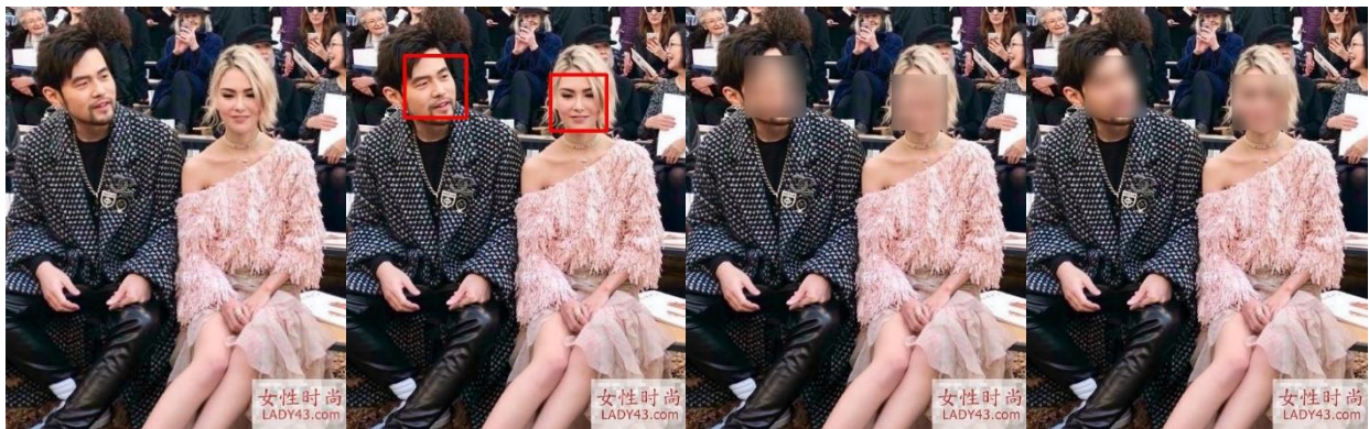
Figures 32-35: From left to right: Original image, faces detected and boxed in, faces box blurred w/ kernel size 45, faces gaussian blurred with kernel size 45 [1]
