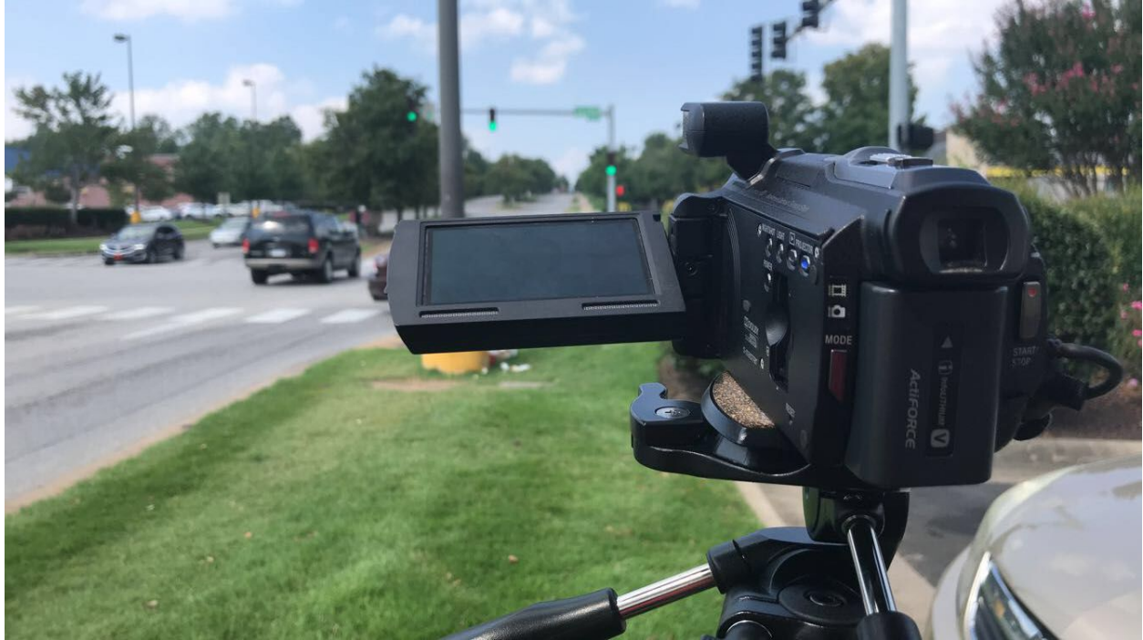
Figure 1. Camera setup used to record the stop lights.
