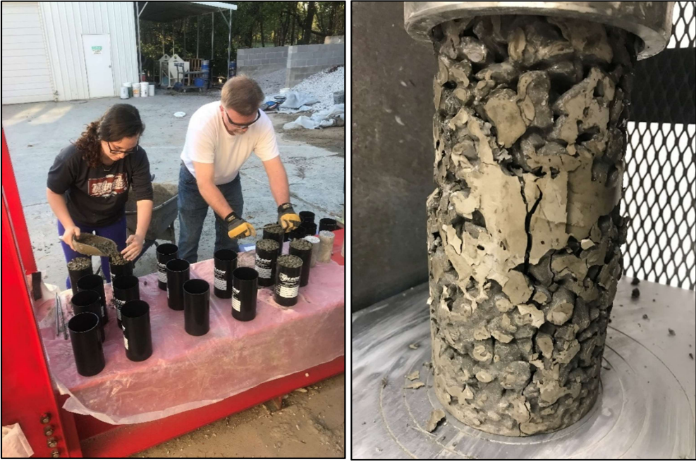
Figure 3. Batching and Testing Pervious Concrete Cylinders
