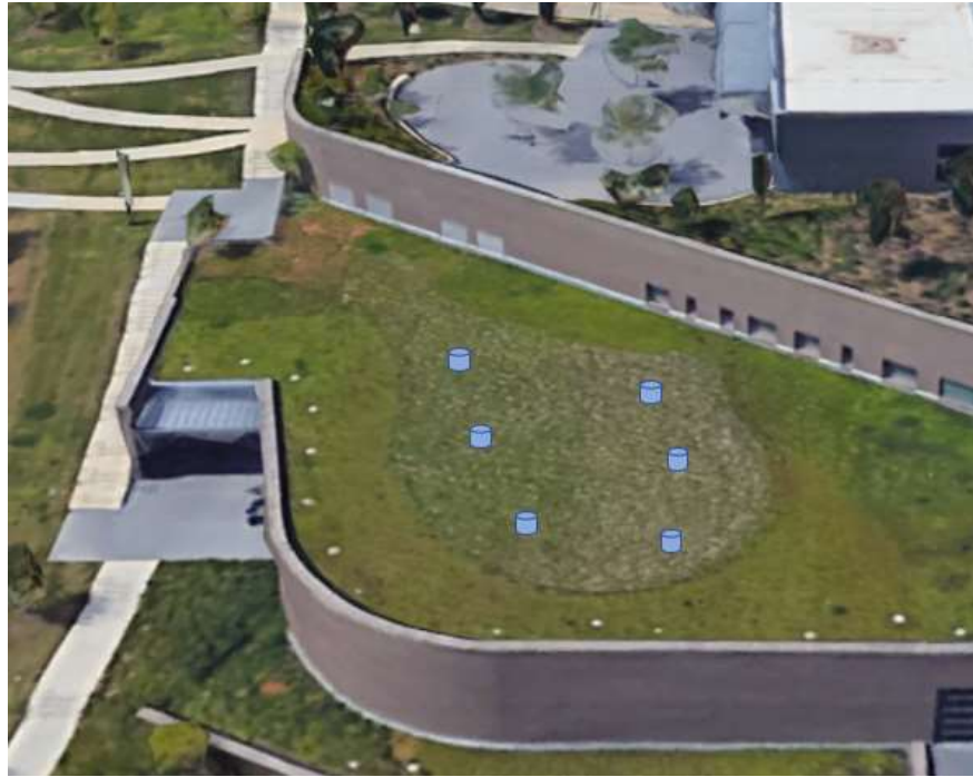
Figure 1. Placement of soil collars on the Hillside Auditorium green roof. Photo adapted from Google Earth (accessed April 15, 2019).
