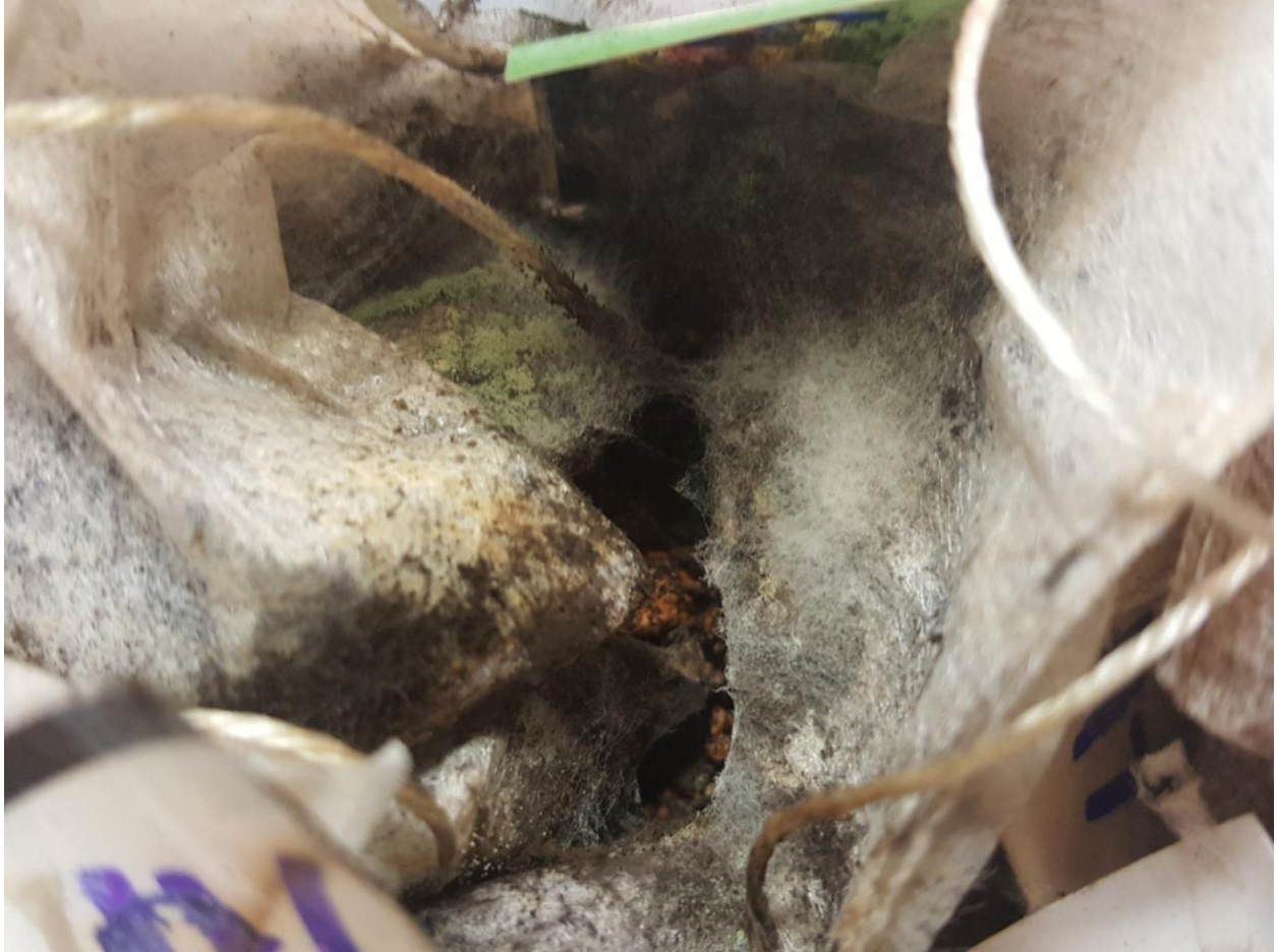
Figure A6: Mold Growth Noted on Tea Bags after Approximately 30 Days of Laboratory Incubation
