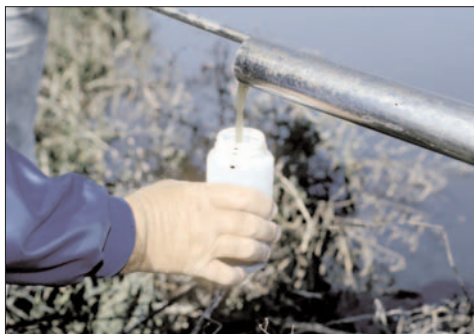
Figure 7. Care when collecting and handling water testing samples assures the integrity of the sample, avoids contamination during sampling, and assures changes do not occur in the sample after it is collected. Precise sampling procedures should be obtained from the laboratory that will be running the tests to assure appropriate samples. (Photo courtesy of USDA/NRCS)
