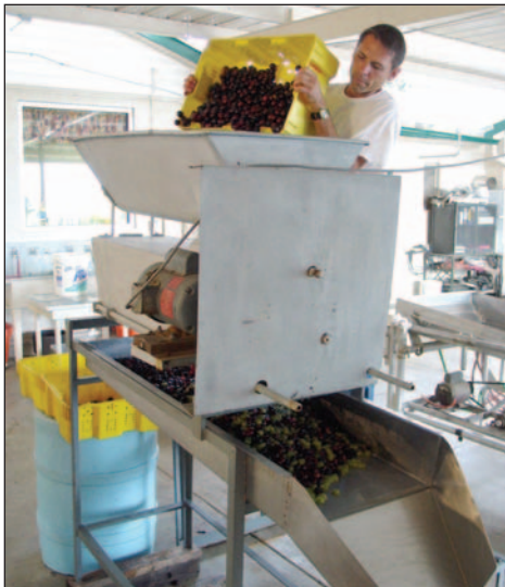
Figure A-3. A crusher is used to break the muscadines so that the juice can be drained.
