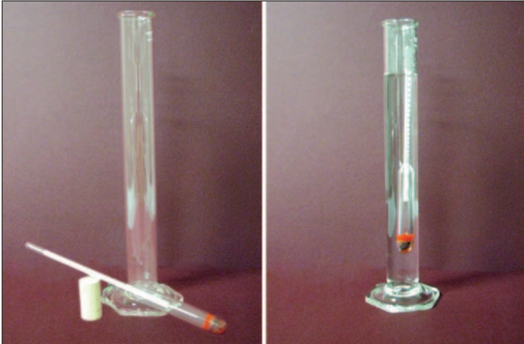
Figure 12. In order to use hydrometers, a sample of juice or wine is placed in a glass cylinder (usually a laboratory graduated cylinder). When the hydrometer is placed in the sample, it will float indicating the amount of material dissolved in the liquid sample.
