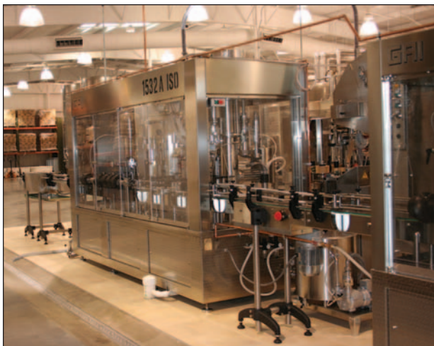
Figure 8. Fully automated bottling lines fill and cork the bottles before moving them directly into labeling machines. (Photo courtesy of Prospero Equipment Corp.)
