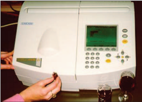
Figure 16. Spectrophotometric analysis is useful for determining turbidity (cloudiness) and ripeness of tannins in wine and juice.
