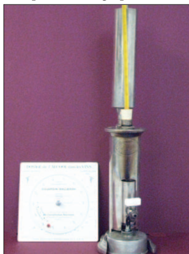
Figure 10. An ebulliometer is used for testing alcohol content of wine. This test is important not only for determination of wine composition but also for tax determinations that are based on alcohol level.
