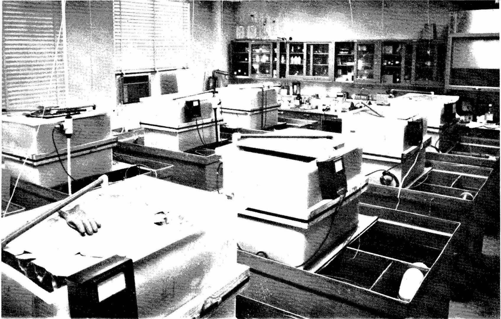
Fig. 2. Siphon and settling basin areas of recirculating systems.
