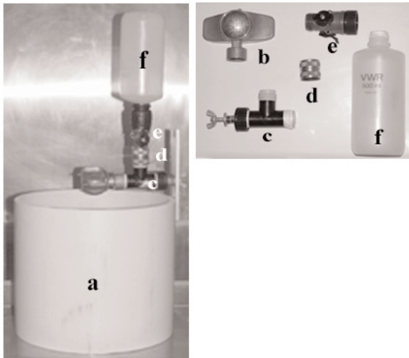
Fig. 1. Treatment applicator developed to apply liquid treatments used a 25 cm diameter PVC pipe (a); a garden hose sprinkler (b); three garden hose adaptors (c, d, e), one of which had an on/off switch (e); and a 500 ml bottle (f). The sprinkler system was set at a height of 10 in.
