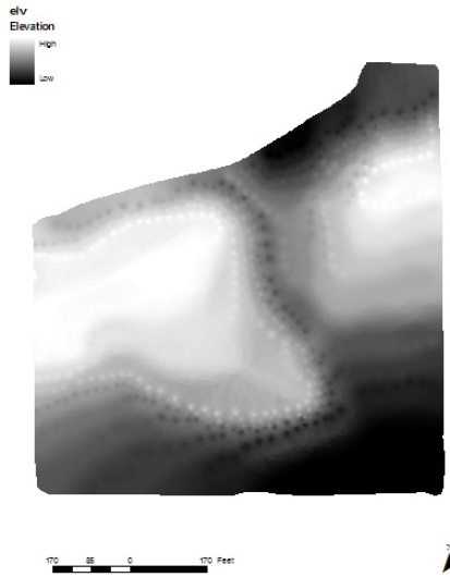
Fig. 1. Elevation surface created by digitizing the levee images.
