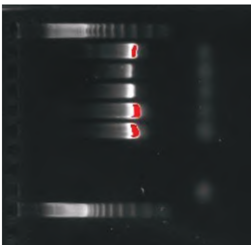
Figure 5: Gel electrophoresis image showing the successful amplification of DNA extracted from biofilms in the pipe samples from the pipe loop on March 22, 2017. The wells contain: ladder, 5 DNA extracts from Galvanized Steel, Copper Type K, Lead, PEX-A and PVC pipes, negative control, and ladder (in vertical order).
