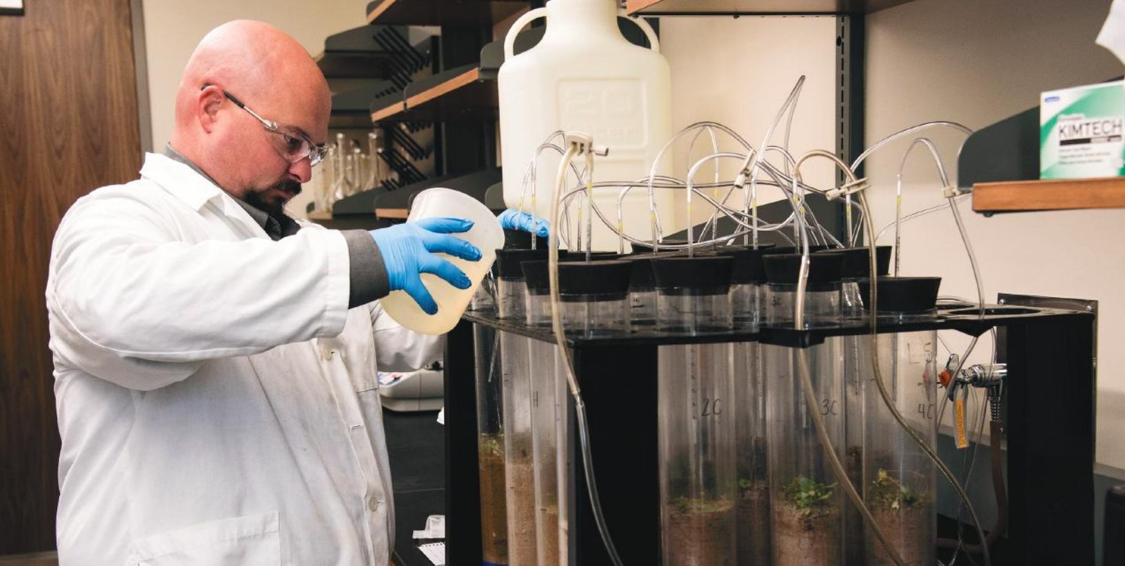
Image caption: Brad Austin, postdoctoral research associate, conducts a sediment experiment using cores collected from a lake. Austin works under the guidance of Center director, Brian Haggard.
