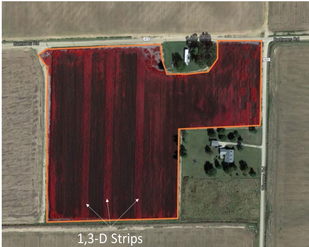
Figure 10. Near infrared (NIR) map at 20-centimeter resolution of a field near Backgate, Arkansas on 3 September 2016 was collected with a multispectral sensor attached to an airplane, showing an elevated level of photosynthetic activity in the three 1,3-D treated strips as opposed to the rest of the field. Higher crop densities are characterized by bright red areas, while dark red to black areas indicate lower crop densities.
