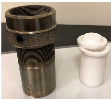
Figure 5.2: The autoclave chamber (left) and the Teflon liner (23mL) (right).
