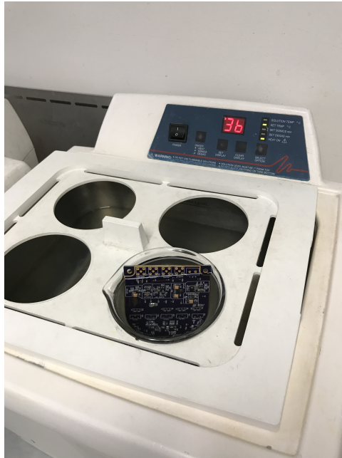
Figure 73: Ultrasonic cleaning of the PCB using 99% isopropyl alcohol.
