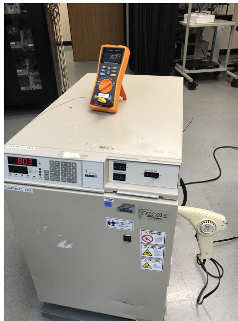
Figure 72: Environmental chamber modified to work as reflow oven.
