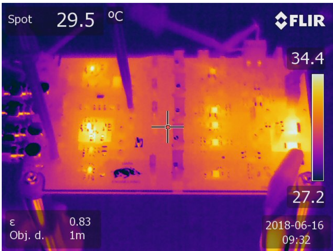
Figure 76: Thermal image of PCB on startup.
