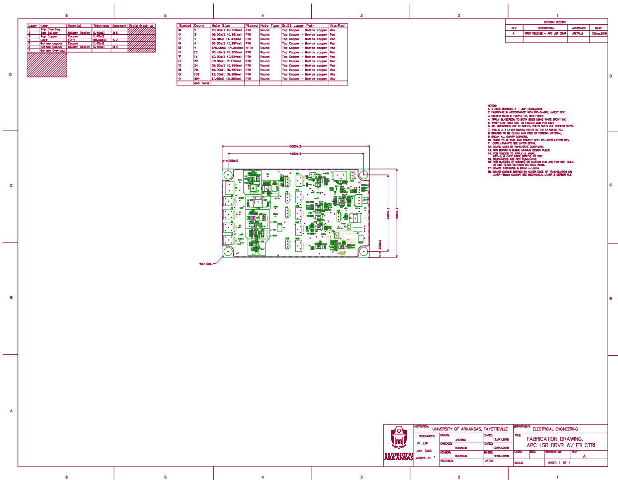
Figure 61: Drawing of the PCB to provide information regarding bare board fabrication.
