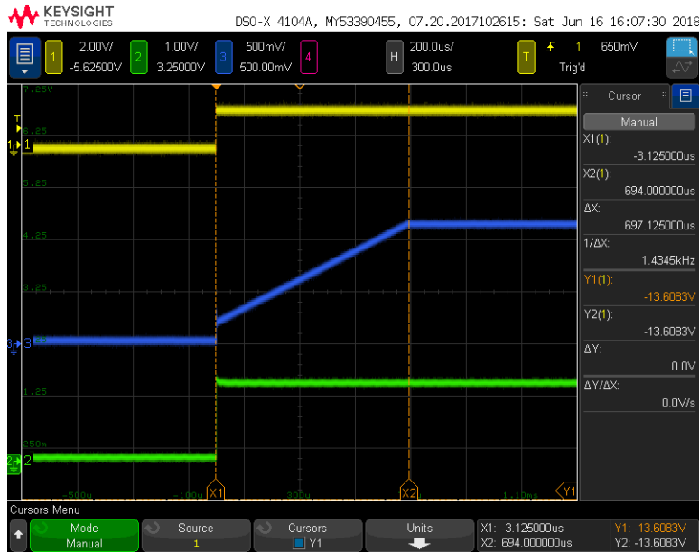
Figure 84: APC PID laser driver settling time to an output disturbance change in set point.
