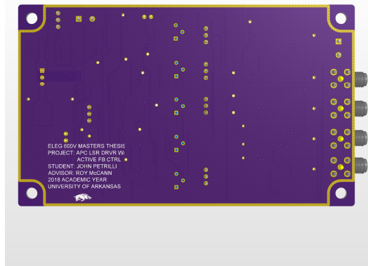
Figure 63: 3D rendered bottom view of the PCBA using Altium Designer 2017.
