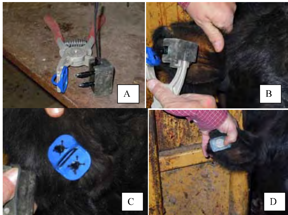
Fig. 1. A) FeverTag before (with applicator), B) during, and C) and D) after application.
