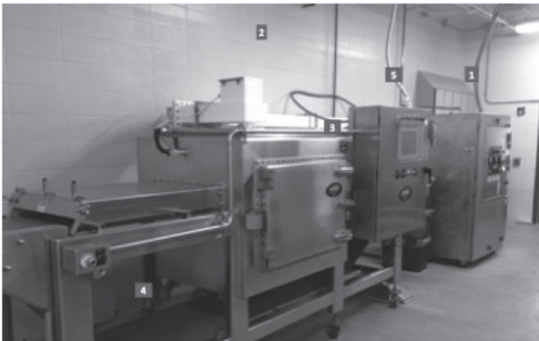
Fig. 1a. Diagram of microwave system showing the transmitter (1), heating zone (2), wave guide (3), conveyor belt (4), and control panel (5).
