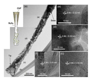
FIG. 1. (Color online) [(a)-(e)] HR-STEM images of carbon/silicon nitride hybrid nanowire. A stacked cone structure of graphitic layers with 0.34-nm spacing is observed at the tip, and the Si<sub>3</sub>N<sub>4</sub> single crystal rod is also seen with 0.66-nm spacing. A schematic drawing of the nanowire structure is shown in the inset of (a).
