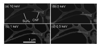
FIG. 3. Series of SE-dominated SEM images of carbon/silicon nitride hybrid nanowire with different beam energies of (a) 10, (b) 5, (c) 1, and (d) 0.5 keV. The CNF tip is in contact with the lacey support.
