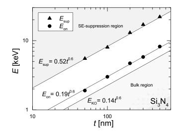
FIG. 8. Si<sub>3</sub>N<sub>4</sub> thickness (*t*) dependence of the three characteristic energies, the onset energy  $E_{on}$ , the suppression energy  $E_{sup}$ , and the Kanaya–Okayama energy  $E_{KO}$ .  $E_{on}$  and  $E_{sup}$  are extracted from the Monte Carlo results in Fig. 7.  $E_{KO}$  is the minimum energy for penetration obtained from Eq. (1).
