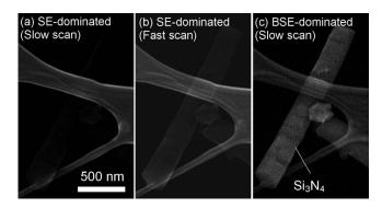
FIG. 5. The signal and scan-rate dependence of the SEM contrast of the  $Si_3N_4$  nanowire with 30 keV beam: (a) SE-dominated image with a single slow scan (20 s), (b) SE-dominated image with multiple fast scans (40 ms/frame, 128-frame averaging), and (c) BSE-dominated image with single slow scan (20 s).
