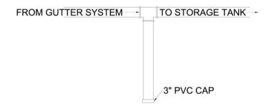
Figure 9: First flush system design.
