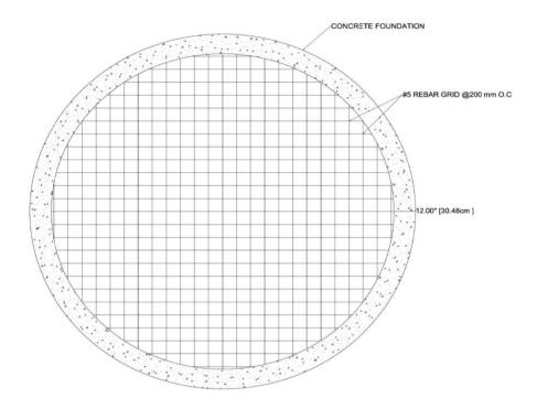
Figure 6: Rebar grid layout.
