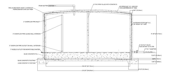
Figure 5: Cross-section of ferrocement tank design.
