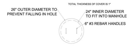
Figure 7: Manhole cover detail.
