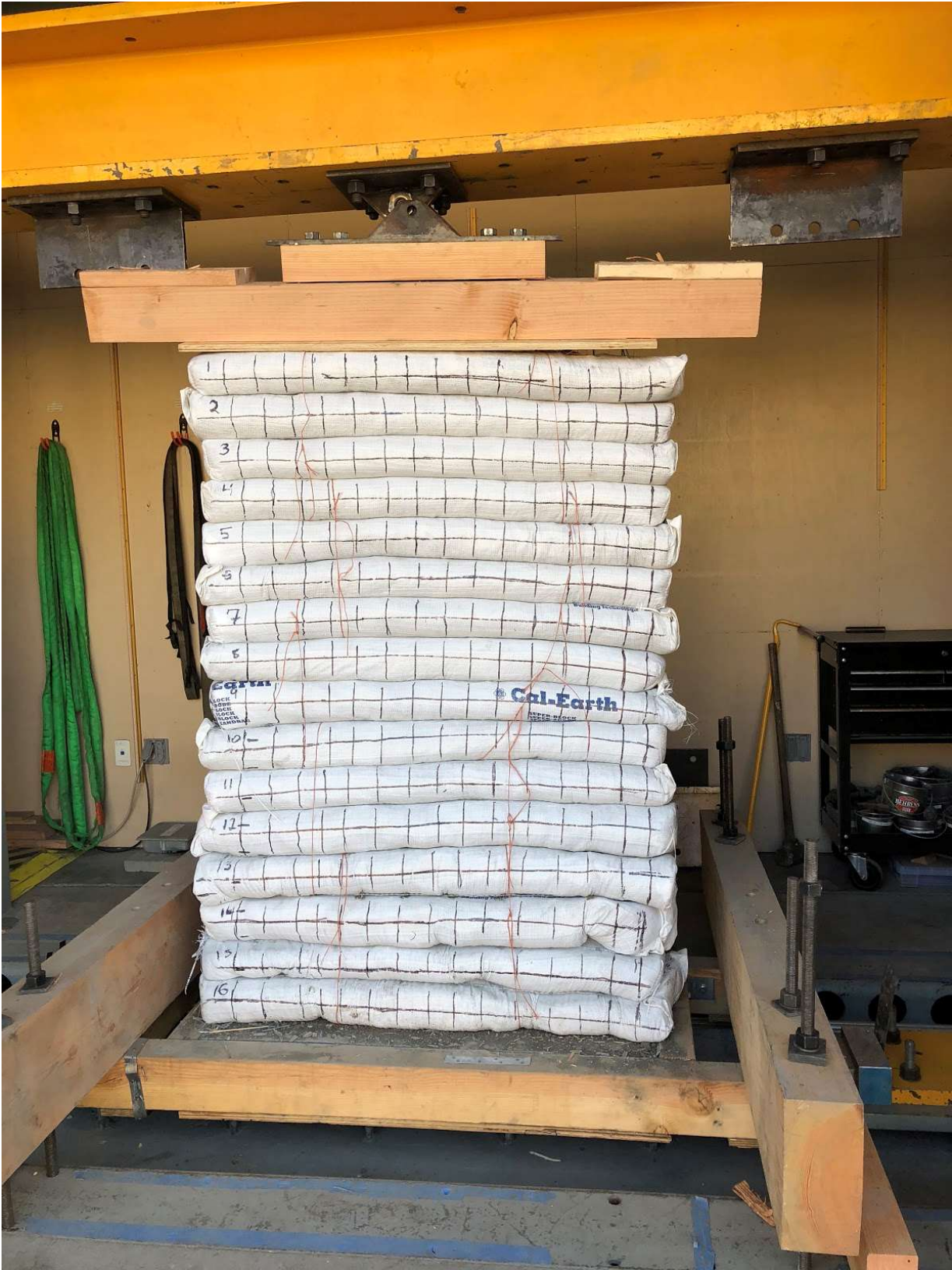
Movement Observed at Top Courses for Wall 1
