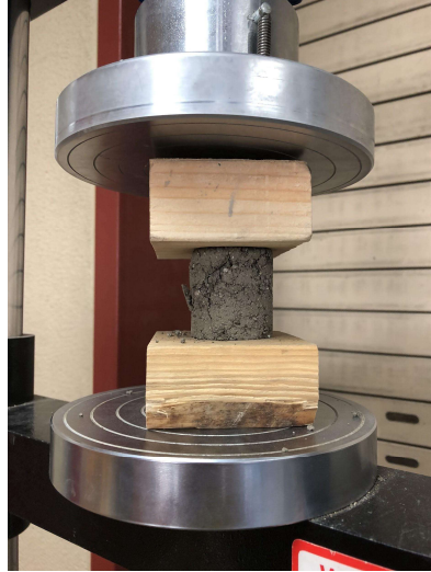
Figure 2: Setup of soil compression tests.
