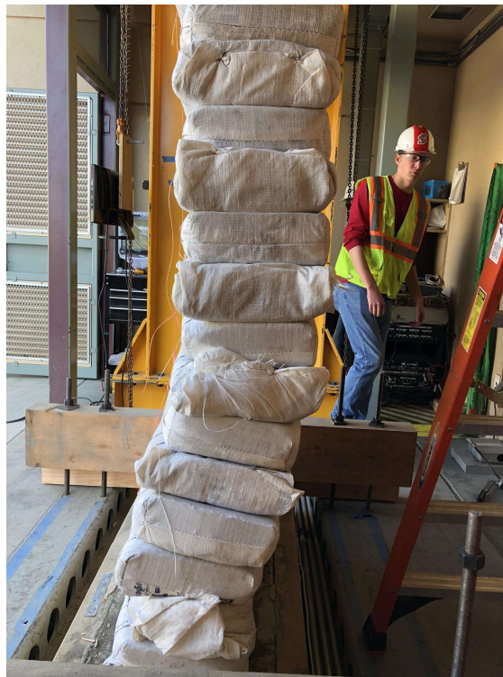
Figure 19: Out of plane buckling of Wall 1.
