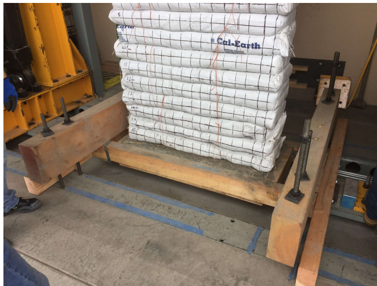
Figure 5: Timber beam members laid across base and connected to strong floor.
