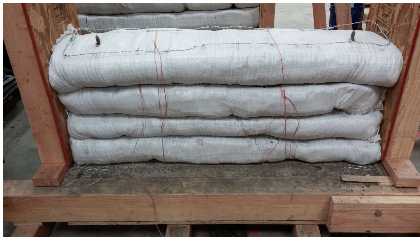
Figure 12: Standard barbed wire configuration between layers.
