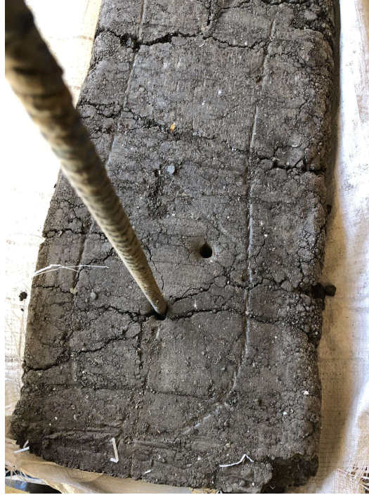
Figure 22: State of soil around rebar lap splice, Wall 2.
