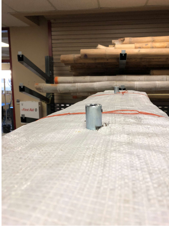
Figure 10: Rebar coupler to threaded rod connection.
