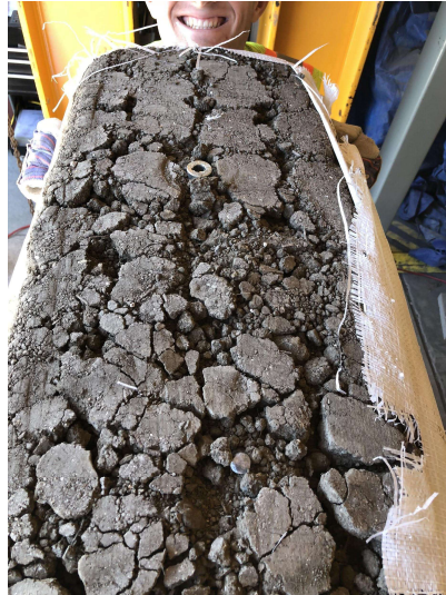
Figure 28: Crushed soil found at the top layer and bond beam interaction, Wall 2.
