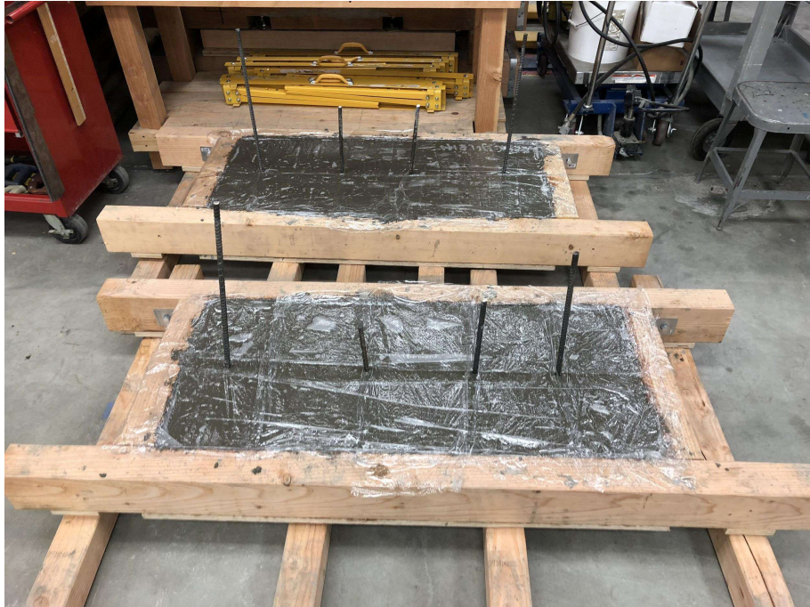
Figure 4: Finished concrete in completed bases.
