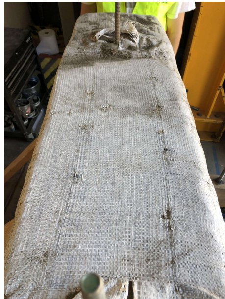
Figure 23: Marks left by barbed wire placed, Wall 1.
