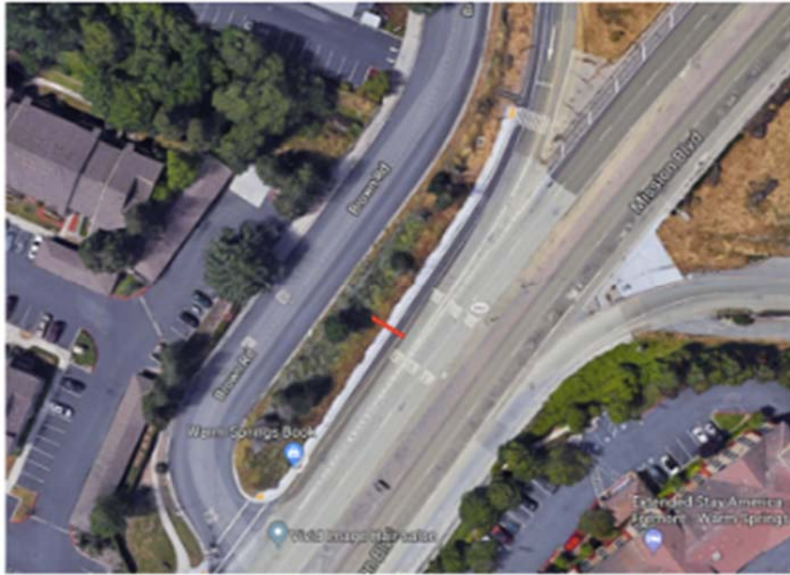
Figure 6: Bird's eye view of existing conditions at merge segment. Red line indicates what will be taken out to account for ramp lane addition.
