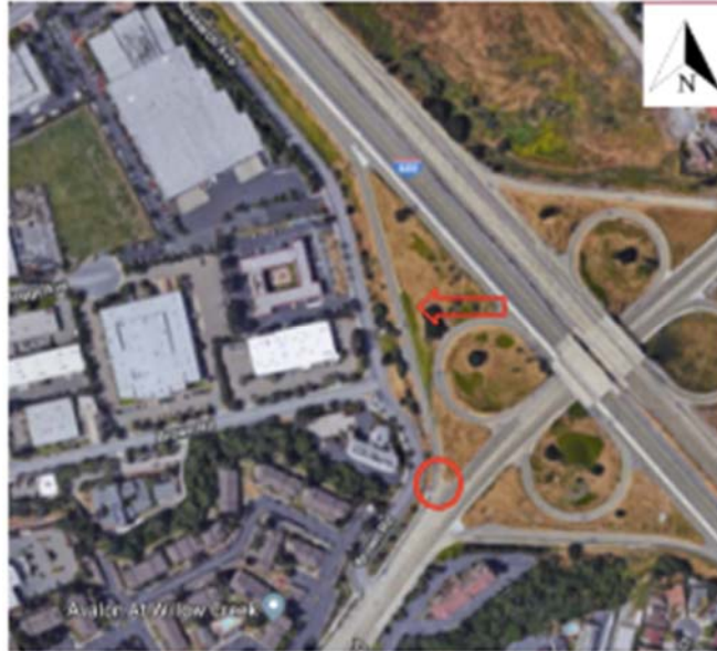
Figure 5: Merge segment from 680 South to Mission West circled in red on four clover leaf interchange, addition of lane location in red arrow.
