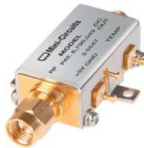
Figure 20: a picture of the power detector used[21]
