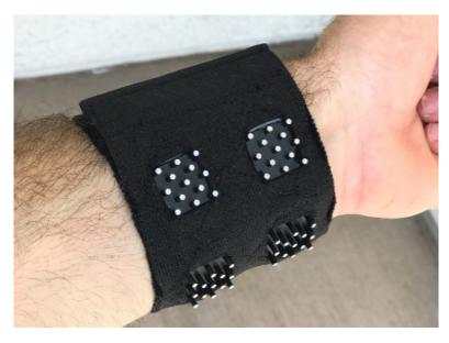
Figure 6: Wristband prototype with integrated TEMs.
