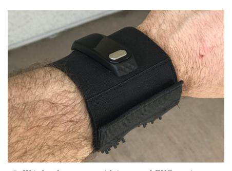
Figure 5: Wristband prototype with integrated EKG monitor on topside.
