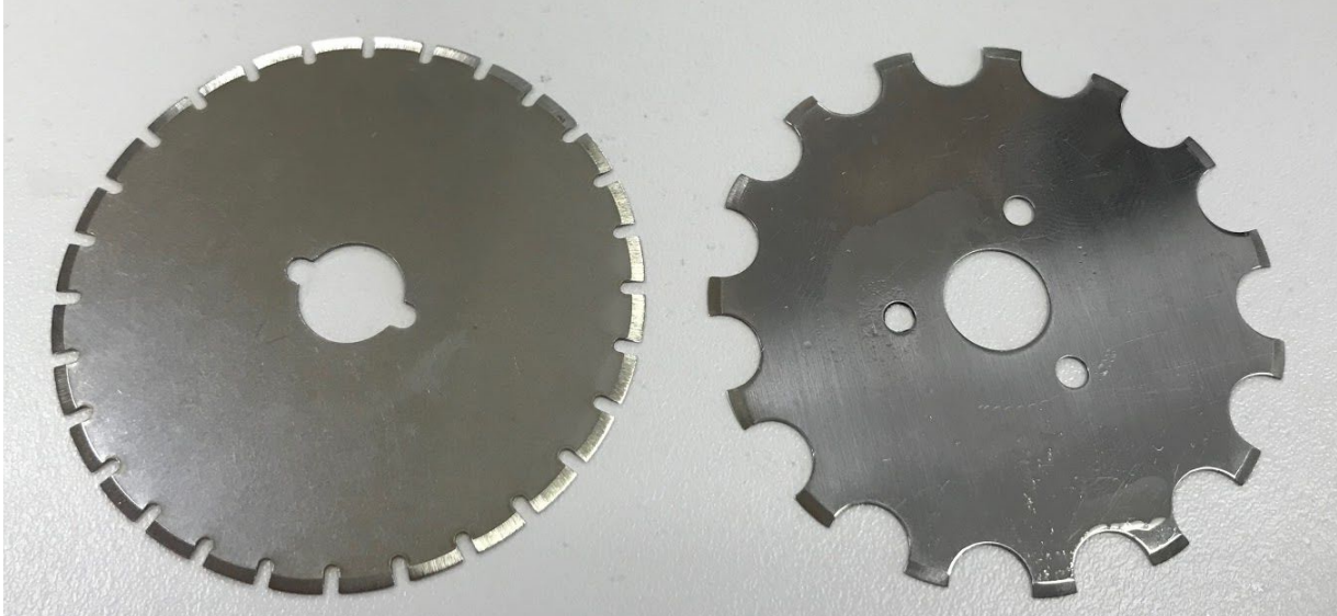
The blade on the left is a 4:1 blade, the one on the right is 1:2.
