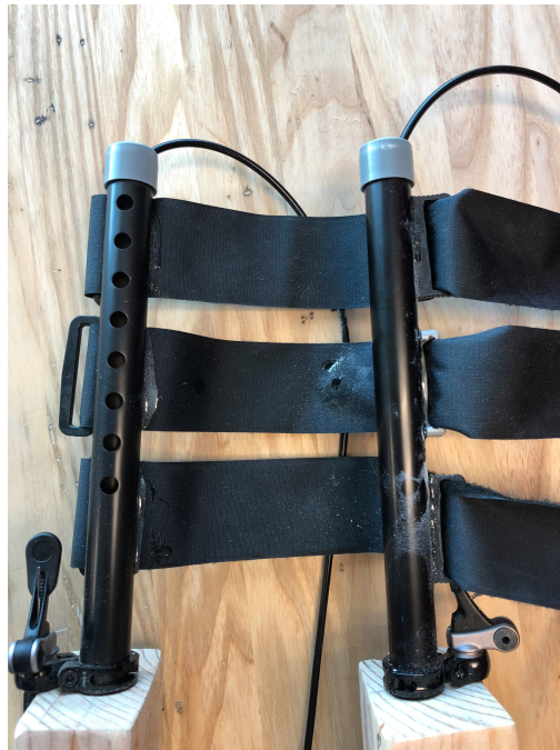
Figure 8: Prototype upper leg frame - dropper post triggers, Velcro straps & buckles
