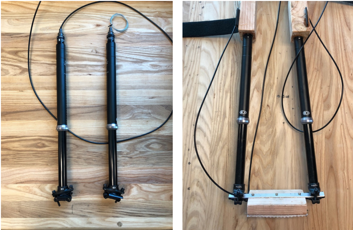
Figure 6: (Left) Dropper Posts, pre-installation Figure 7: (Right) Lower leg frame, post-assembly
